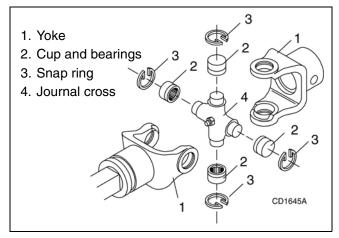
Figure 22. U-Joint Exploded View
